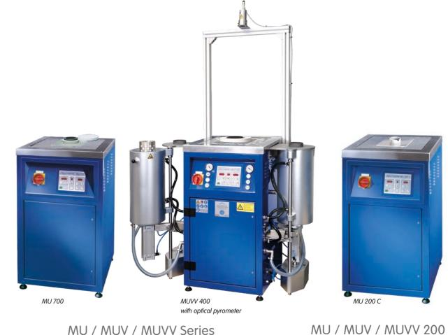
Melting by induction technology: The crucible containing the material is placed in the core of the induction coil. A strong alternating magnetic field generates a strong alternating current in the graphite crucible and in the metal. This results in rapid heating and thorough mixing of the material.
