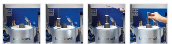
For sintering, the individual layers are centered on a spindle. For the simultaneous processing of multiple rings, the rings are separated by graphite shims.
