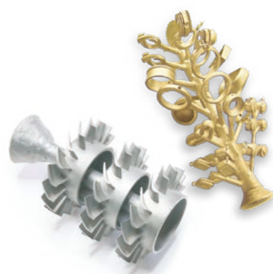
Casting trees in steel and in gold
