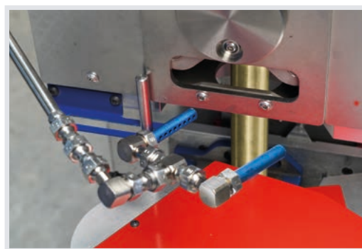
Secondary cooler at the outlet
