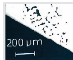
Porosity without vibration
