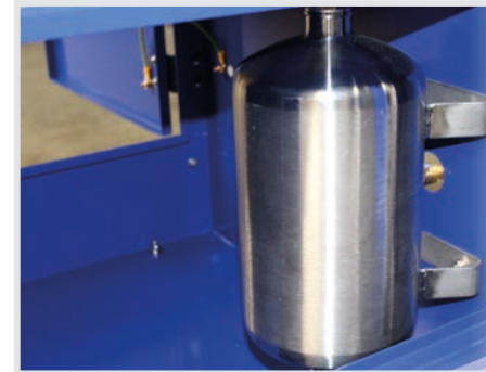
An additional pressure tank integrated into the plant provides for even faster pressure build-up for activation of the Turbo Pressure PLUS function.
